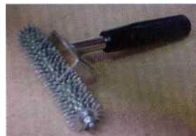
10-889 Carpet Seam Roller 15cm Used to blend fibres when seaming carpet.
